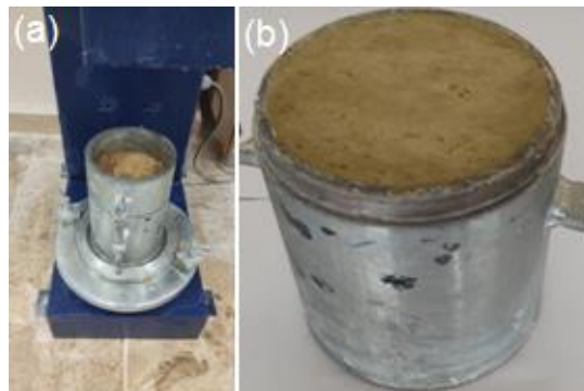
Visual 3. Performing the standard proctor experiment (a), compressed sample as a result of the experiment (b).
