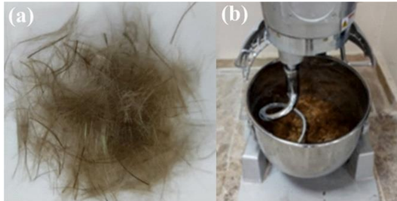
Visual 2. Compressor separated BF (a) and preparation of clay and BF mixtures (b)
