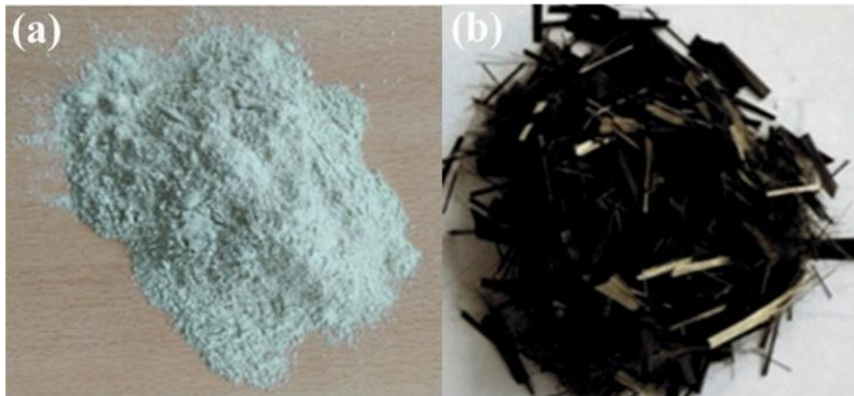
Visual 1. Bentonite clay (a) and unseparated basalt fiber (b) used in the study
